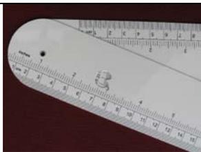
The scaling is in cm and inches. Through an eye in the longer arm one can see the scaling for angles from 0-25 degrees on the shorter arm.
