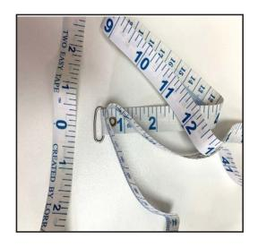
Example of the two measuring tapes, showing the '0' (zero point) of the Two Easy tape and the loop end of the Companion Inseam tape. The Companion tape slides onto the Two Easy tape and allows you to take inseam and crotch length measurements all at one time.
